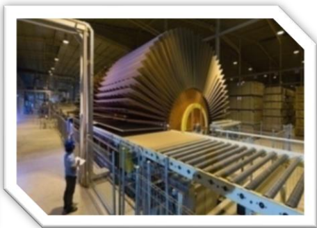
COOLING STACKING & HANDLING SYSTEM
